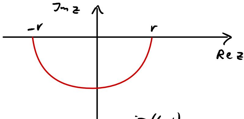
$$\text{parametrization } \varphi(t) = r e^{i\pi(t-1)}, \quad \varphi : [0,1] \rightarrow \mathbb{C}$$
