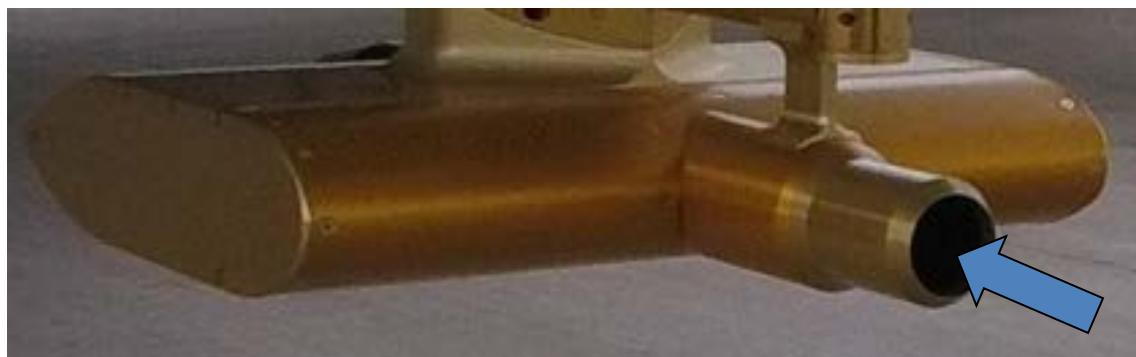
Measured particle size: 0.51 - 50  $\mu\text{m}$
