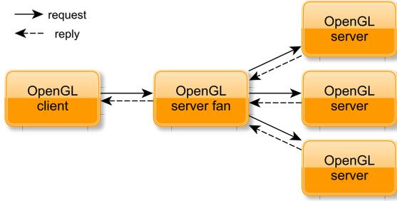
(a) Traditionally, the client's requests are fanned to the distributed renderer and replies are merged after a full round trip. The display's semantics and pragmatics are opaque to the client.
