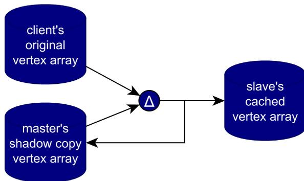
Figure 4: Vertex Array Cache – The master maintains a shadow copy of the client’s vertex arrays. The vertex array transmission to the slave is differential.
