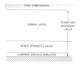
Viscous layer Friction by molecular viscosity: relative motion at the surface is zero, and viscous media resist shearing
