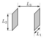
To investigate this, we consider in the following two conducting plates with surface areas  $A = L_1L_2$  separated by a distance  $L_3$ . In the plane of the plates we will still be using periodic boundary conditions and con-
